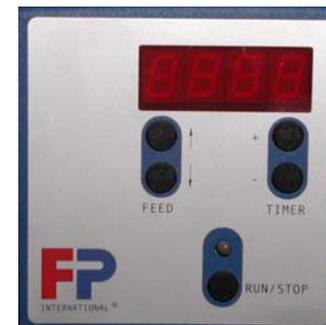
**Setting the type of production cycle** By pressing the upper FEED-↑ (B) and TIMER + (C) key shortly, a choice can be made between a production cycle of a certain time (seconds) or length (meters). If length is chosen, an L will appear in the left side of the display\*\*.
